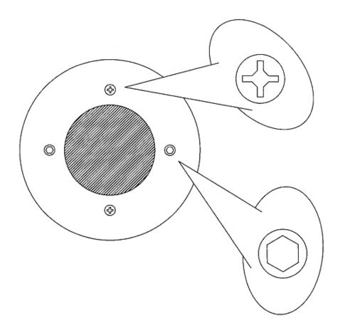
To remove the spot, unscrew the two screws with cross-shape cut. Then, to dismount the stainless steel ring, unscrew the two screws with hexagonal-shaped head. In mounting the spot, please use opposite proceedings, and assure to clean and correctly place all components (gasket, glass, nuts, ring and screws). At the end close strongly the screws with an appropriate tool.
